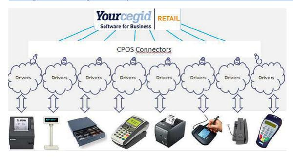
Instead of exchanging directly with each device, the POS terminal now communicates with a generic multi-device connector called CPOS.
